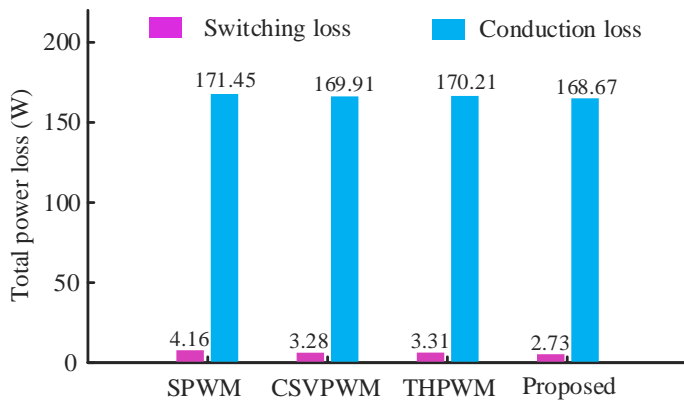
Fig. 7. Total power loss comparison among different PWM techniques for unity modulation index.
